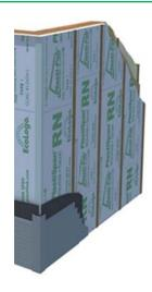
PlastiSpan® RN insulation applied to the exterior of above-grade wood frame walls is a great way to increase the energy efficiency of that portion of the home. PlastiSpan RN insulating sheathing is manufactured with the long edges routed out to fit a  $19 \times 64$  mm ( $1" \times 3"$ ) nailer. The recessed nailer provides a flat surface for the installation of exterior cladding.
